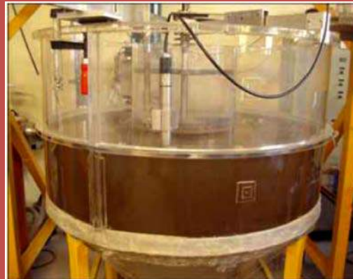
Annular flume (to study about sediments)
