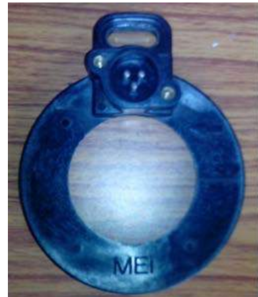
Brake wear sensor for heavy vehicles
