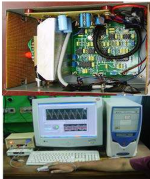
Calibration free pulse oximeter
