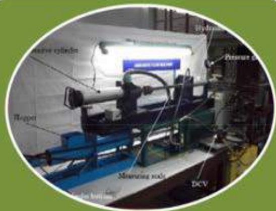
Abrasive Flow Machine for Producing Nano level Finish on Complex and Inaccessible Internal Features
