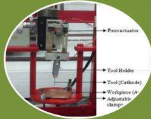
Micro-EDM for Micro-machining of Holes and Channels for Micro Fluidic Applications & New Approach for Nano Particle Generation
