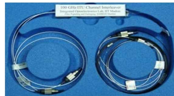
Fiber Pigtailed & Packaged DWDM Channel Interleaver (100 GHz)
