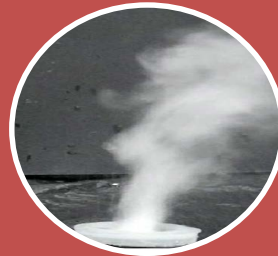
Ultrasonic atomization for gasoline engines: Low droplet sizes at even atmospheric pressure
