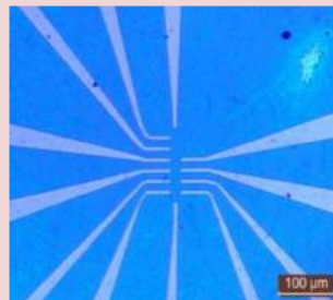
Nanoscale transistor device with electron-beam lithography
