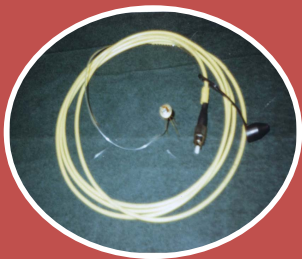
Pigtailed InGaAs/InP p-i-n Photodetector with micromachining for fibre coupling
