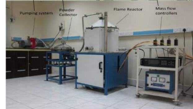
Chemical vapour synthesis set-up (top) Flame synthesis set-up (bottom)
