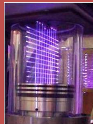
Laser grid inside the engine cylinder
