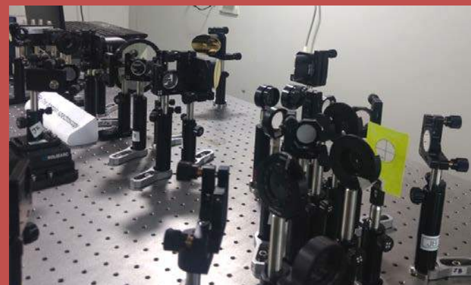
THz time domain spectroscopy set-up
