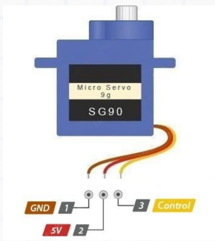
DC Servo motor wiring connection
